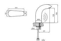
Comfort length: 134 mm Comfort height: 119 mm Electric / battery powered (4x1.5 V AA) (Batteries included) Single water inlet. If desired, constant temperature can be provided with double water inlet by using 410600100603. IP 56 Junction box
